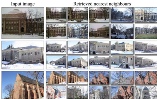
Fig. 3. Some image retrieval results. The retrieved images contain real neighbors of the input image, and some false positive cases as well. The false positive cases can be removed after applying epipolar constraints subsequently.
